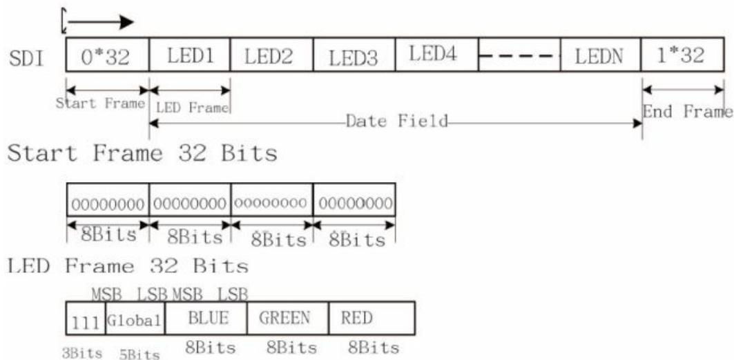
Each update consists of a start frame of 32 zeroes, 32 bits for every LED and an end frame of 32 ones. I am not sure what the “End Frame” is good for, since its encoding is indistinguishable from a LED set to maximum brightness and will simply be forwarded to the next LED. In my experiments, omitting the end frame did not have any impact.
