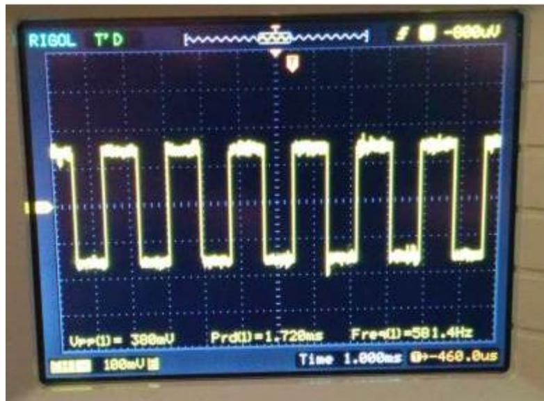
The picture above shows the current modulation for RGB=255,255,255 and the global brightness set to 16 (50%). The pulse width modulation is clearly visible in the voltage signal at a frequency of 580 Hz, very similar to the 430 Hz of the WS2812.
