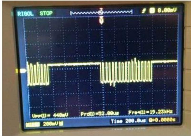
Next, I set the RGB value to 128,128,128 and kept the global brightness at 50%. The result is shown above. Two PWM modulation schemes are superimposed in this configuration. The global brightness is still modulated at  $\sim 582$  Hz, while RGB value is modulated at an approximately 32 times higher frequency, 19.2 kHz. This frequency is significantly above the flicker fusion threshold, even when moving the LED around, leading to an apparent constant brightness.
