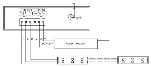
When connect three channels LED, you should put the Dream Color software switch to CD mode to use, only under this mode, you can control the LED's color, brightness and speed. Color disk adjust the color (Adjust process can be seen in the upper left corner R, G, B numerical with change), speed/brightness item adjust speed and bright ("M"set the LED dynamic effect, "M"adjust the LED dynamic change.
