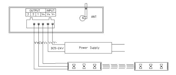
When connect three channels LED, you should put the Dream Color software switch to CD mode to use, only under this mode, you can control the LED's color temperature, brightness and color temperature shortcut key settings. Color disk adjust the color temperature (meanwhile top left CW,WW numerical with change), brightness item adjust bright, "M"key set the special color temperature state.
